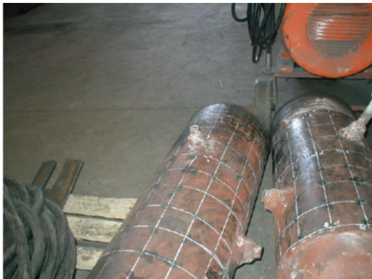
Figure 5-8 Boiler feed lines removed because of flow-accelerated corrosion
