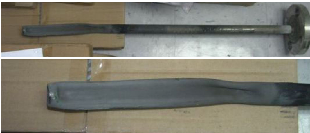
Figure 3-12 Collapsed Kanthal 2 protection tube caused by external pressure
