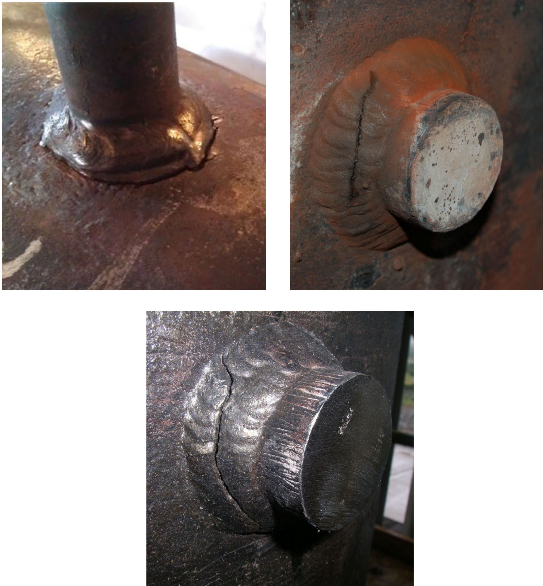
Figure 8-2 Typical RT-plug weld failures
