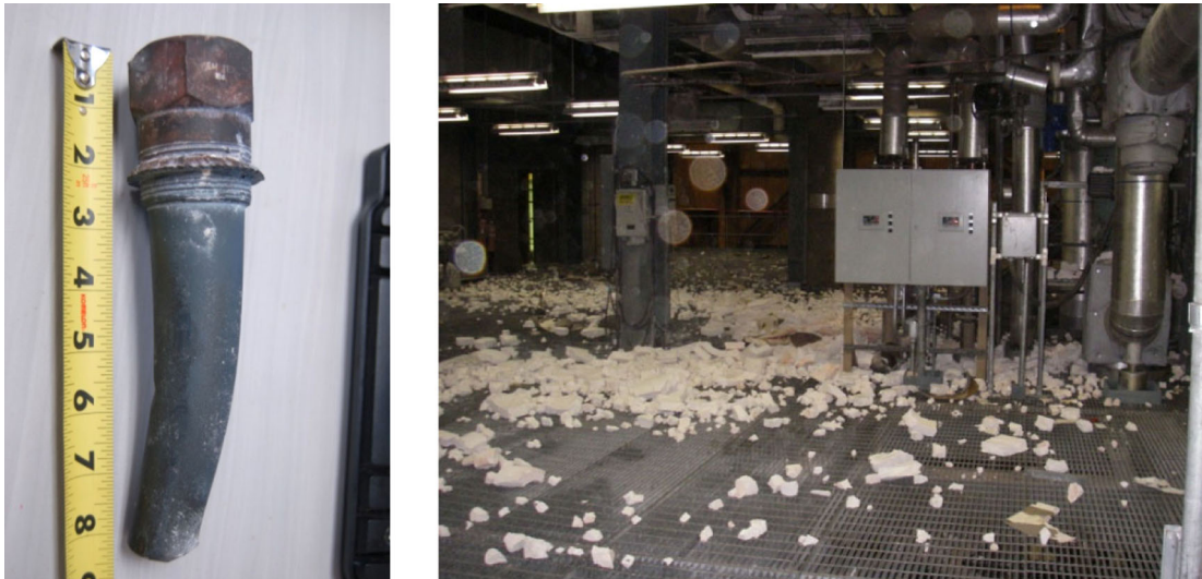
Figure 5-3 Ejected thermowell (left) and the damage (right) caused by the thermowell ejection
