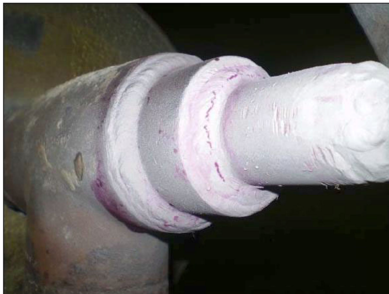
Figure 5-5 Installed thermowell exhibiting unsafe cracking at the weld
