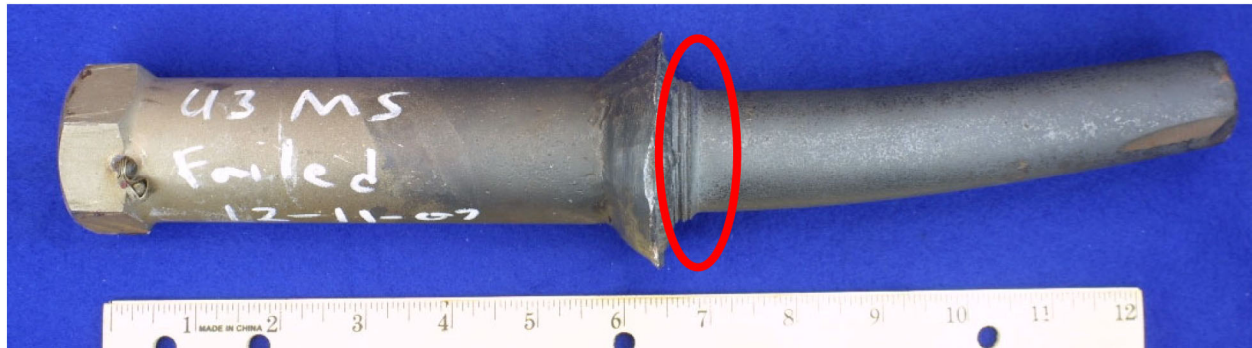
Figure 5-1 Thermowell retrieved following ejection from a main steam line
