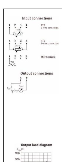
8N is a basic, programmable non-isolated, easy-to-use 2-wire transmitter. The Low Profile housing has a hight of only 18.5 mm / 0.72 inch. Configuration is made in seconds with the user friendly Windows software. No external power supply required for configuration. The transmitter is programmable for RTD's in 3- and 4-wire connection according to different standards as well as for 11 T/C types.
