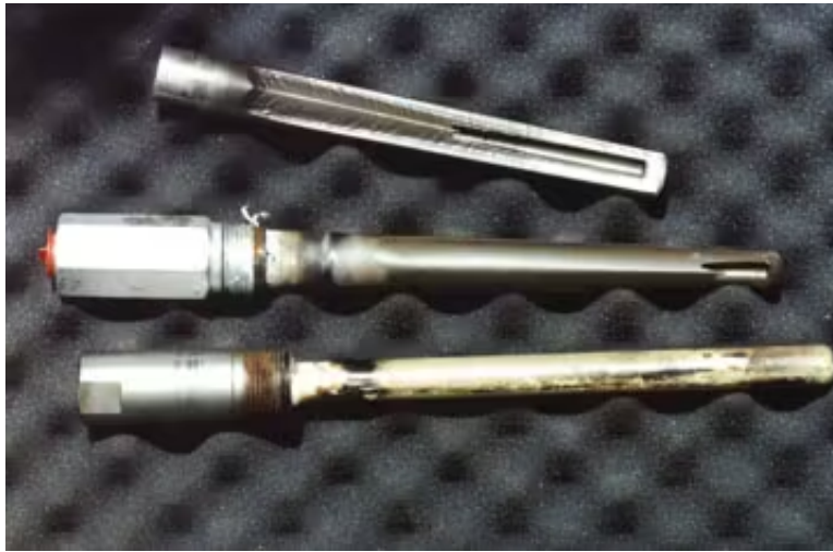
Figure 1. The top two thermowells failed open due to corrosion in coal pulverizing line despite cobalt hard face coating. The protection tube on bottom survived without failure despite longer exposure in process.
