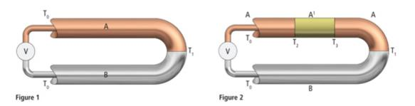
Note the difference in the Seebeck coefficients for the two conductors appears in Equation 3. This always happens in thermocouple loop analysis, and it is the property that is of practical interest in thermocouple thermometry. It is called the relative Seebeck coefficient (between material A and material B) and is written "S<sub>AB</sub>." That is,
